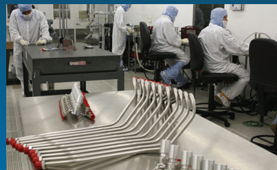
Complex Ultra-High Purity Gas Delivery System Assembly
